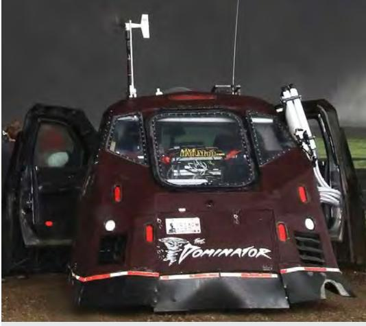
THE DOMINATOR AND DATA-COLLECTING INSTRUMENTS MOUNTED ON THE DEBRIS-RESISTANT ARMOR, WAITING FOR INTERCEPT OF A LARGE WEDGE TORNADO. USED WITH PERMISSION.
