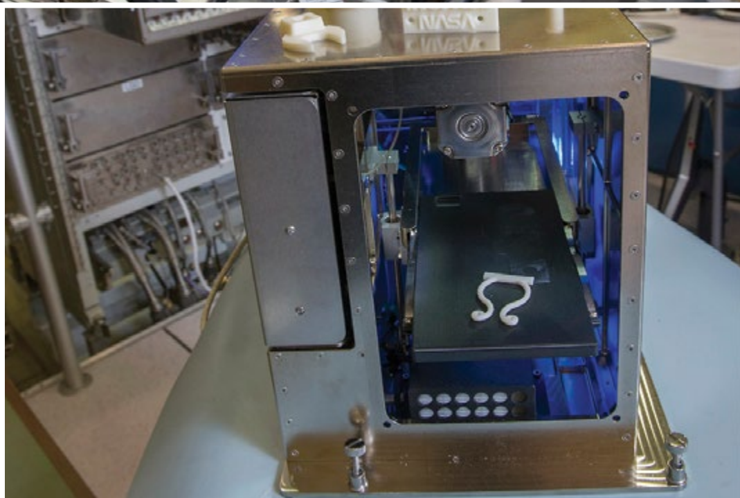
THE 3D PRINTER USED ON THE INTERNATIONAL SPACE STATION. PHOTO COURTESY OF NASA. USED WITH PERMISSION.
