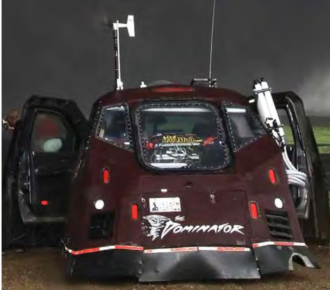
THE DOMINATOR AND DATA-COLLECTING INSTRUMENTS MOUNTED ON THE DEBRIS-RESISTANT ARMOR, WAITING FOR INTERCEPT OF A LARGE WEDGE TORNADO. USED WITH PERMISSION.
