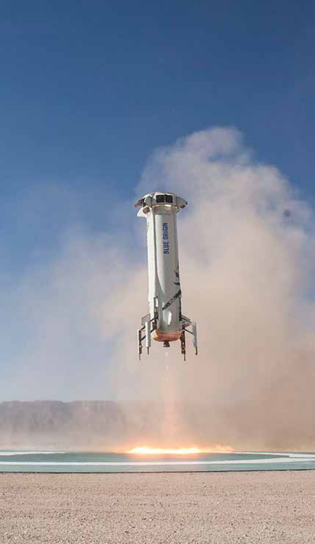
BEZOS' "NEW SHEPARD" ROCKET RETURNING TO ITS LANDING PAD AFTER A QUICK JAUNT TO SPACE.
