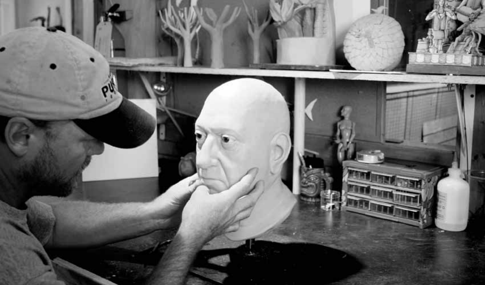
An artist puts the final touches on a clay sculpture. It will be used to mold silicone skin for an animatronic character. Used with permission.
