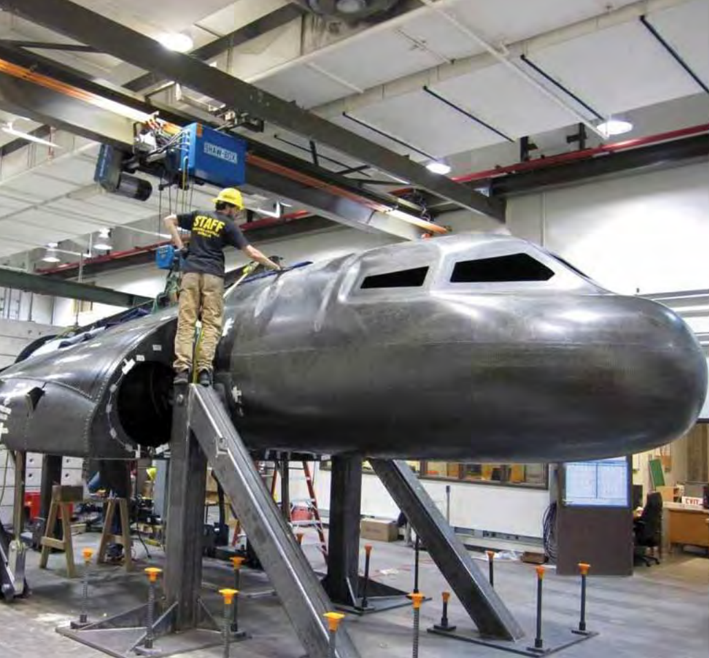
Dream Chaser structural test article. Used with permission.
