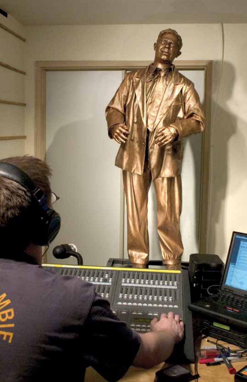
A control technician programs a character move by move in synchronization to the audio presentation. Used with permission.
