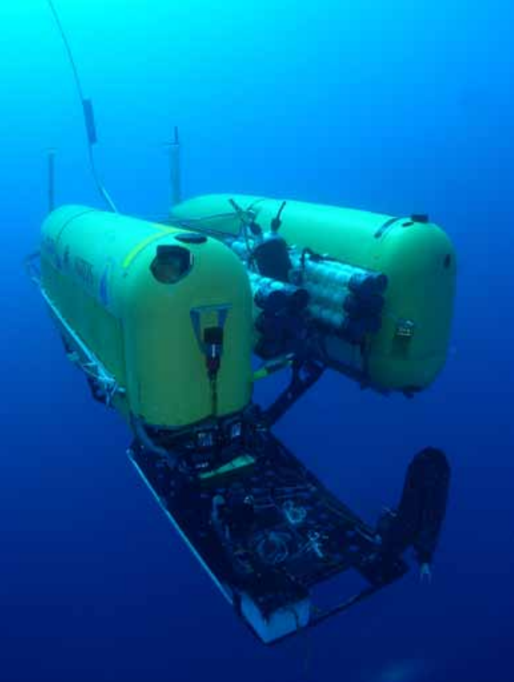
The hybrid remotely operated vehicle (HROV) Nereus is a one-of-a-kind vehicle that can operate either as an autonomous, free-swimming robot to conduct wide-area surveys, or as a tethered vehicle for close-up investigation and sampling of seafloor rocks and organisms. On its maiden dive in May 2009, the vehicle successfully reached the deepest part of the world's ocean—Challenger Deep in the western Pacific Ocean. During its second expedition in October 2009, it investigated hydrothermal vents along Earth's deepest mid-ocean ridge in the Cayman Trough. In 2013, as part of the newly funded HADES project, Nereus will be used to conduct the first systematic study of life in ocean trenches—the deepest marine habitat on Earth.
