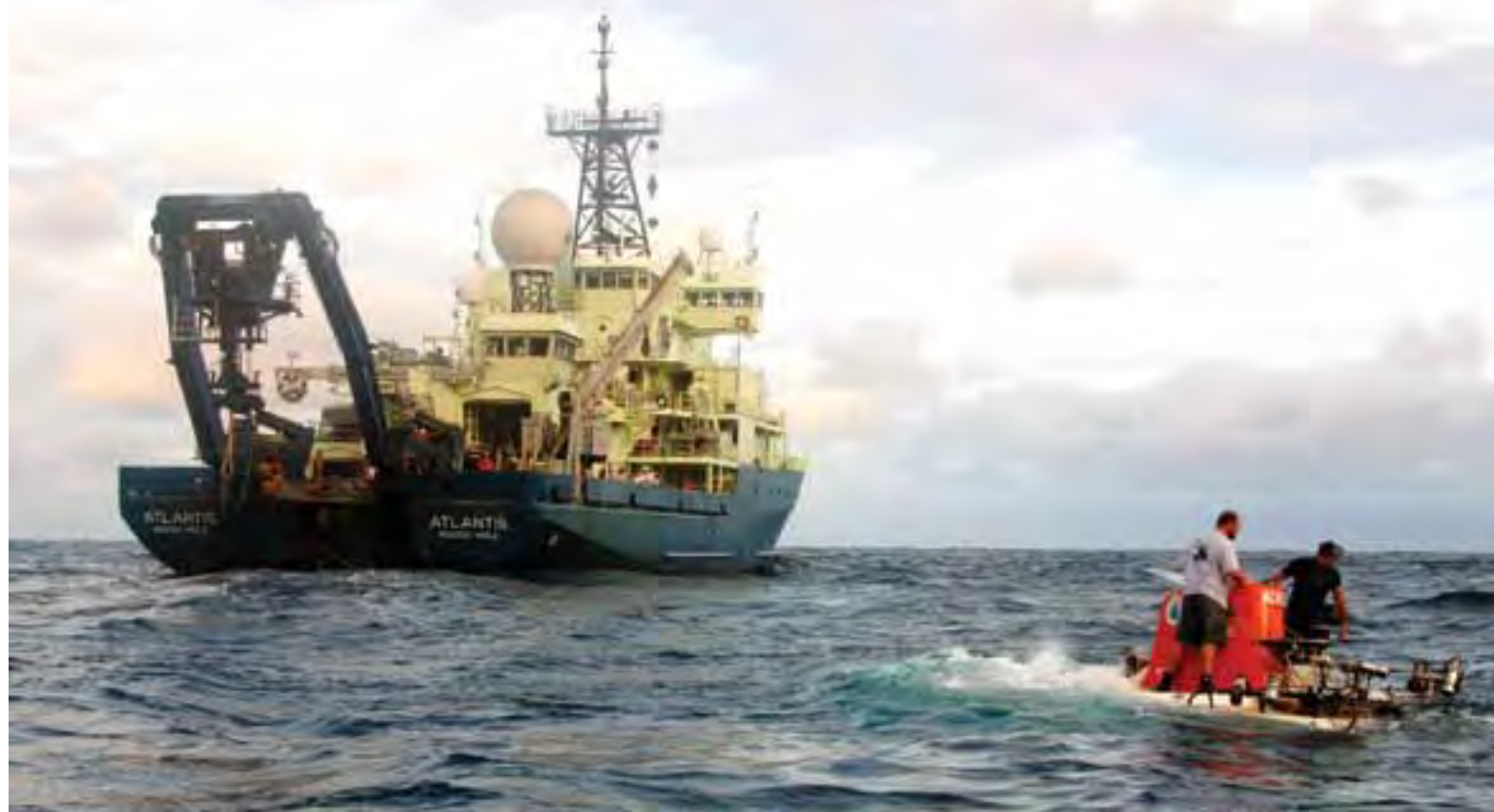
The WHOI-operated research vessel Atlantis serves as support vessel for ALVIN operations. During each recovery, two certified swimmers help bring the submersible back to the ship. Photo by Amy Nevala, Woods Hole Oceanographic Institution. ©Advanced Imaging and Visualization Laboratory, Woods Hole Oceanographic Institution
