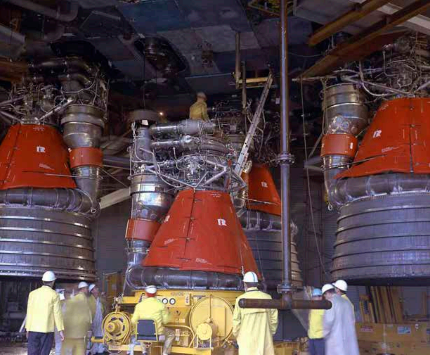
TECHNICIANS INSTALLING ONE OF FIVE F-1 ENGINES AT THE BASE OF THE SATURN V'S FIRST STAGE. CREDIT: NASA.
