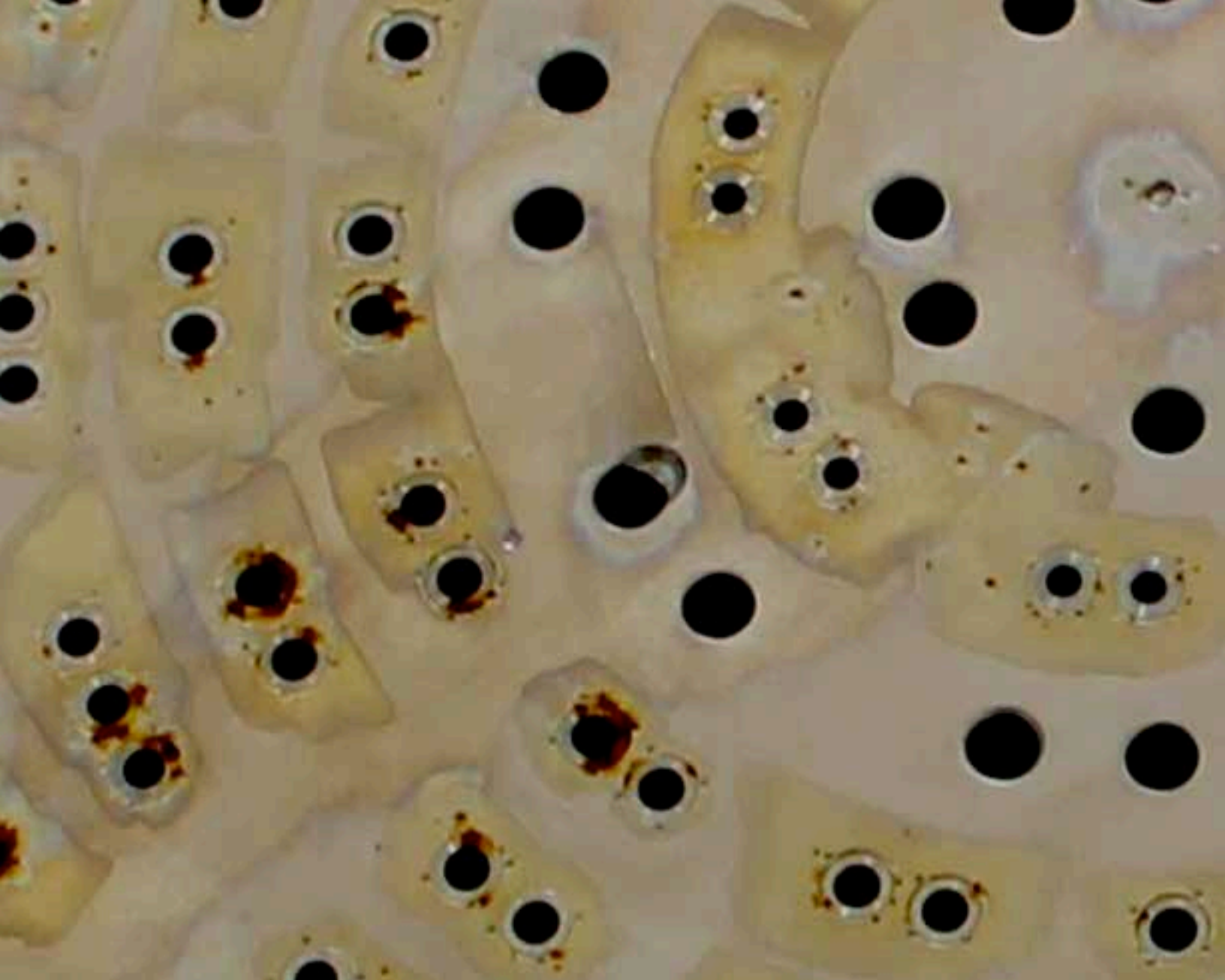
CLOSE VIEW OF THE F-1 FUEL INJECTOR PLATE. NOTE THE NUMEROUS ABORTED DRILL MARKS, WHERE INJECTOR HOLES WERE STARTED, THEN ABORTED. IT WAS ENGINEERING BY TRIAL-AND-ERROR. CREDIT: NASA.
